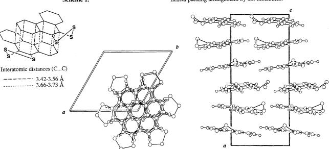
**Figure 1.** The crystal packing of trithiole **1c**. Selected bond lengths (Å), bond angles(°), and torsion angles(°) are as follows: S-C 1.789(5), 1.778(5); S-S 2.063(2), 2.052(2); S-S-C 93.0(2), 93.4(2); S-S-S 94.92(9); S-S-S-C 40.0(2), -40.8(2). Intermolecular C---C contacts are shown in Figure.
